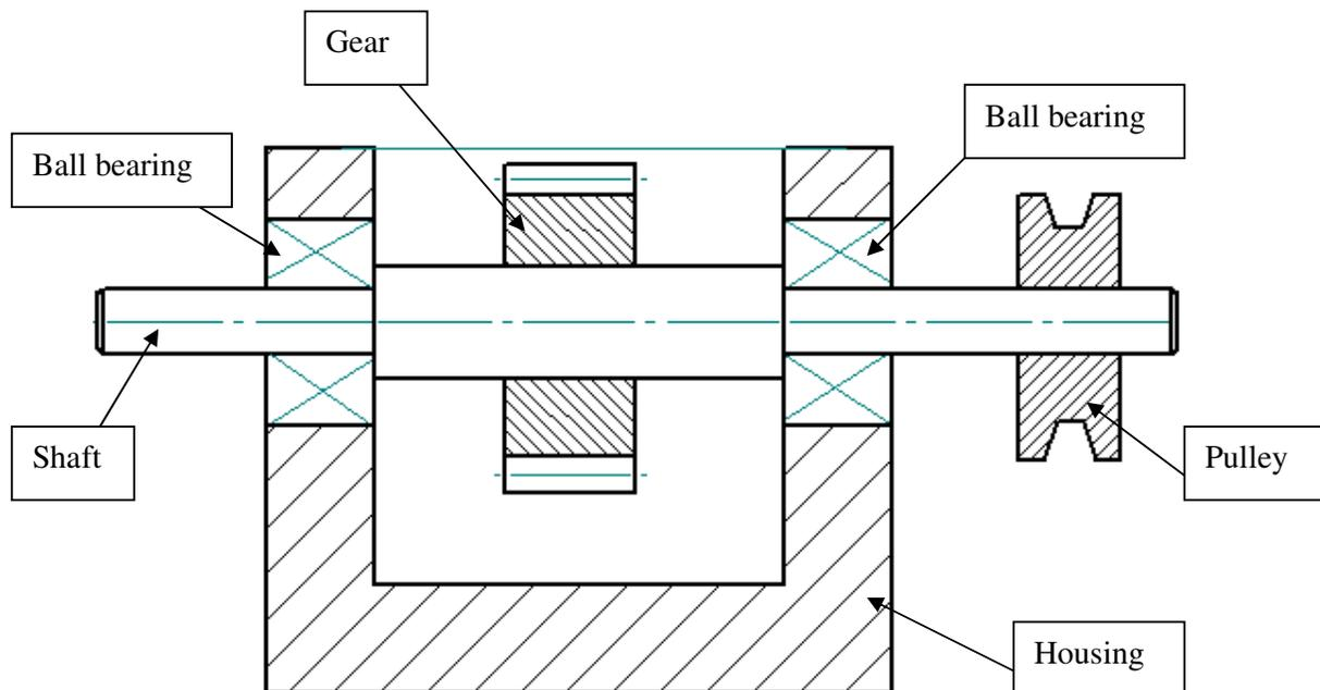
Between ball bearings and shaft is interference fit.
