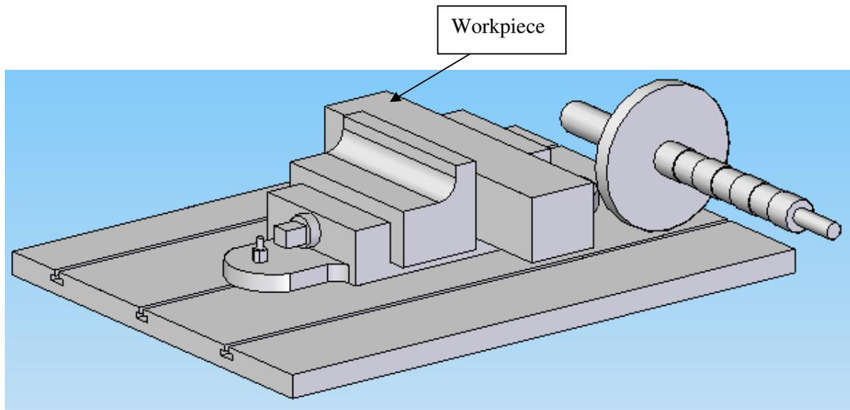
Below are the features of the vice that automatically align the fixed jaw parallel to motion 2 and perpendicular to motion 3.
