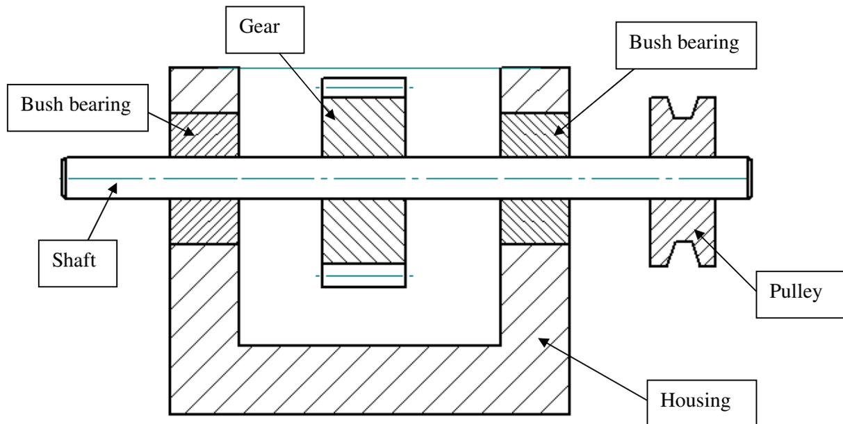
Between bush bearing and shaft is clearance fit.
