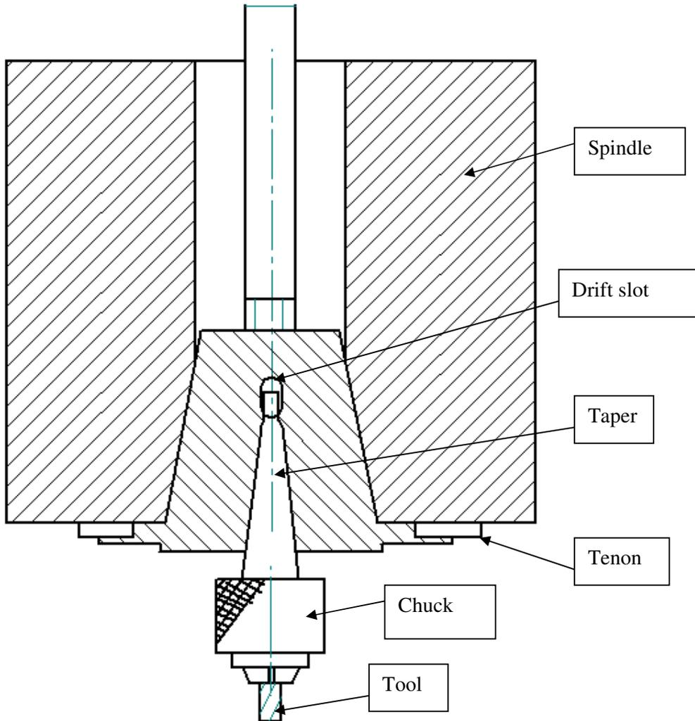
This is a holder, which introduces a standard taper at the spindle nose. The spindle is therefore able to take either a drill directly, or a drill chuck in which a tool is held.
