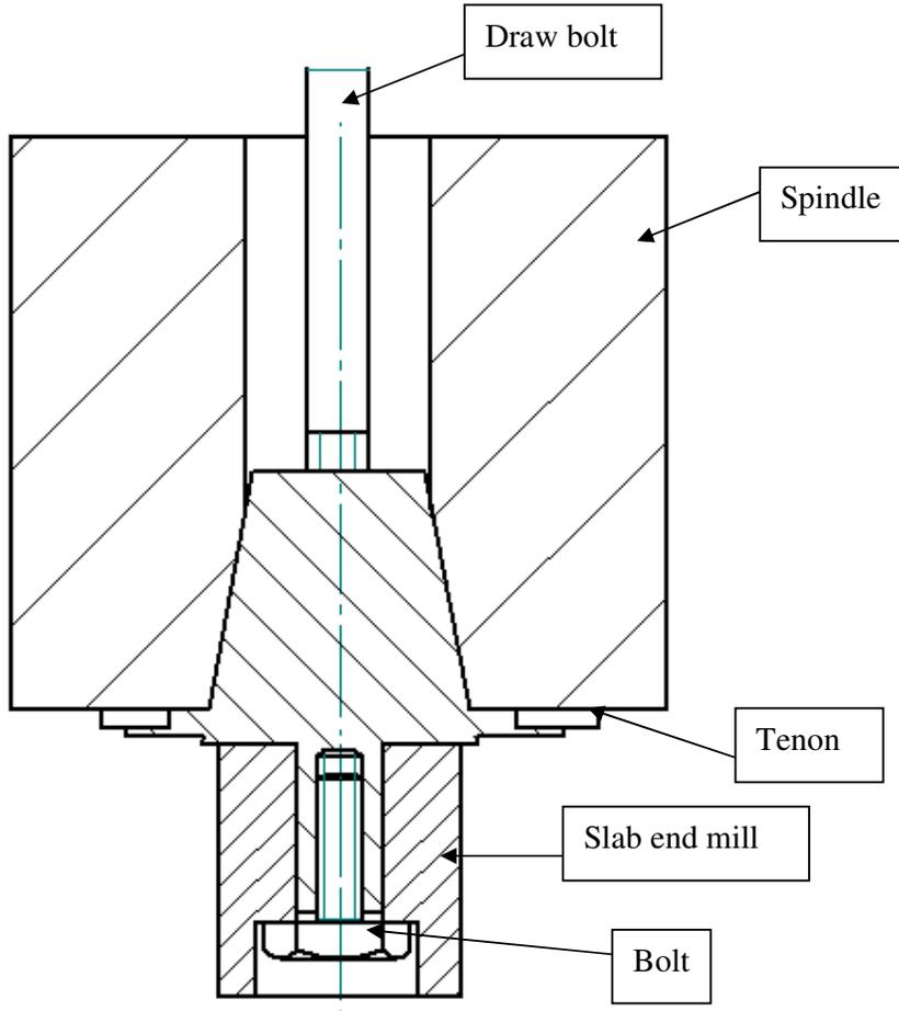
In both cases, the tool is positively held in the holder and therefore can take both axial and radial loads without coming loose due to vibrations from the cutting forces.
